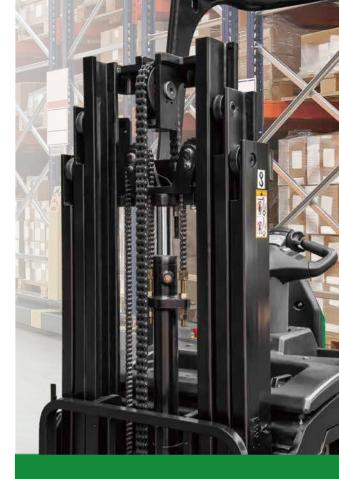
The lifting cylinders have been optimized for design, ensuring stability and reliability, with reduced stress and increased durability.
